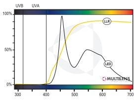
Due to technical constraints for high intensity LED-lights, the typical wavelength curve for these lights looks as above. Our LLR-filter cuts off the peak around 450 nm, which results in less glare and better comfort.
